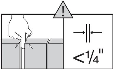
CAUTION: Spacing between boards must be less than 1/4" or a finger entrapment could exist.
